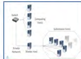
Figure 1: High level design for HPC cluster in Ankabut
