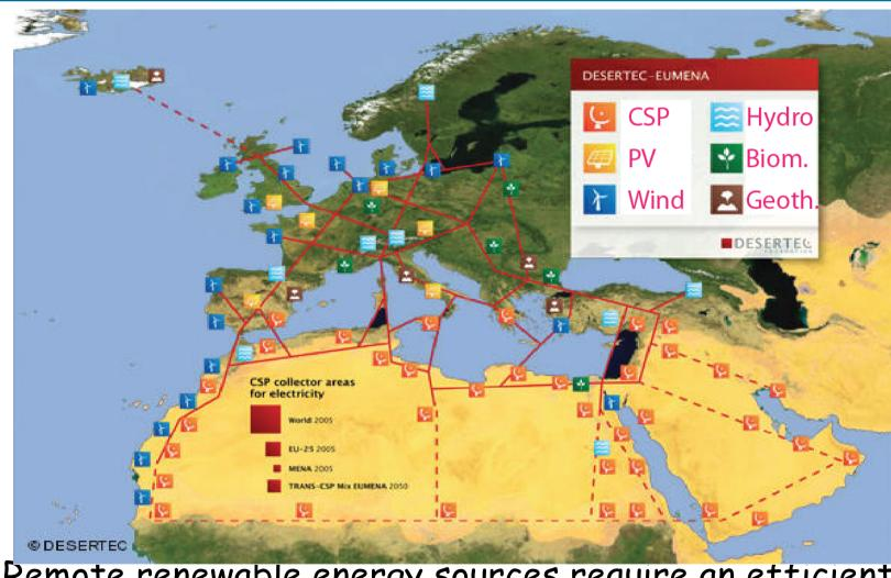
Remote renewable energy sources require an etticient transfer of electrical energy over long distances.
