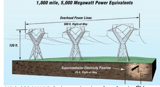
With 800 kV HVDC, the overhead surface for the EU-MENA-2050 lines is 3600 km<sup>2</sup>, to be compared with 2500 km<sup>2</sup> for the CSP plant itself: SC lines are almost a necessity.
